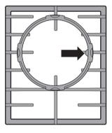
You can use a wok on these burners without any additional rings, trivets, etc.
